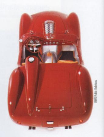
The customers got everything they bargained for, and then some. The Sport Speciale Roadster has a behemoth 5.97L V-12 BMW engine capable of generating 480 foot-pounds of torque and 450 horsepower. The 2,230 pound Sport Speciale can accelerate from 0-60 in 3.6 seconds and has a theoretical top speed of 251 miles per hour! For comparison purposes, the Ferrari from which
